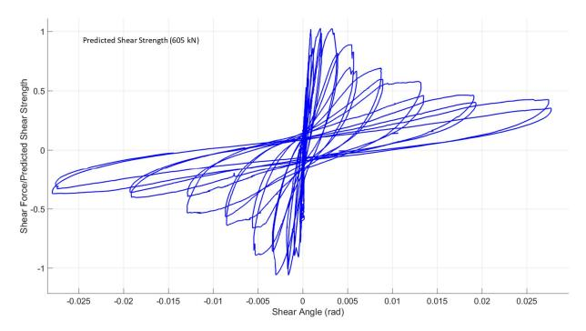
Figure 5. Load Deformation Plot of Specimen 3/6.25-4-L-NF-DT
