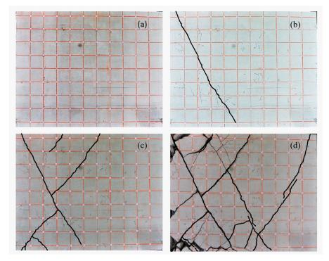
Figure 6. Progression of failure for specimen 3/7.5-4-N-NF-DT. (a) Before testing. (b) First appearance of diagonal tension cracking. (c) First appearance of diagonal tension cracking in opposite direction. (d) Crack pattern past failure
