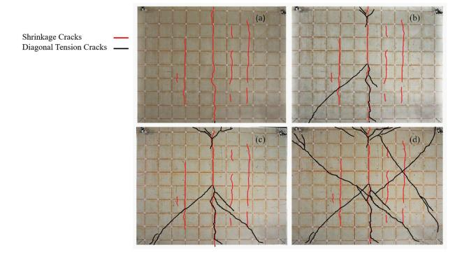
Figure 4. Progression of failure for specimen 3/6.25-4-L-NF-DT. (a) Before testing. (b) First appearance of diagonal tension cracking. (c) First appearance of diagonal tension cracking in opposite direction. (d) Crack pattern past failure
