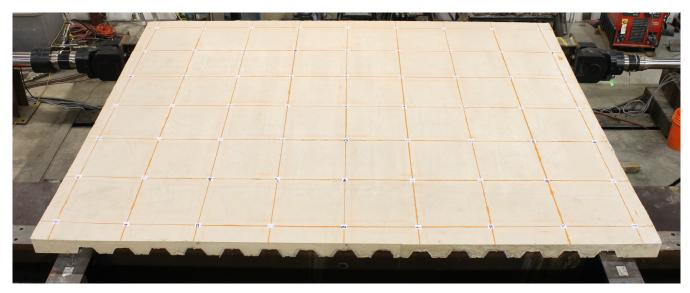
Figure 3. Experimental Setup for Cantilever Diaphragm Tests
