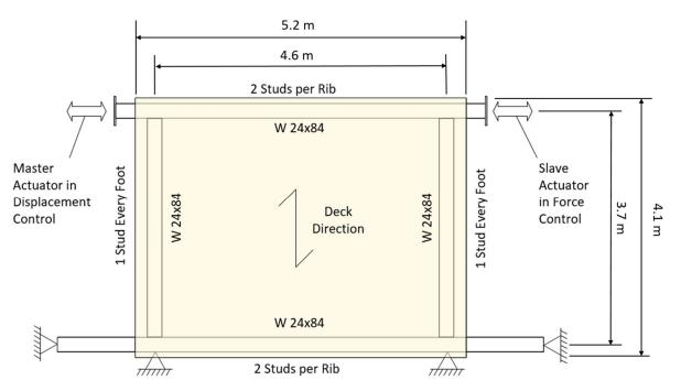
Figure 1. Experimental Setup for Cantilever Diaphragm Specimens
